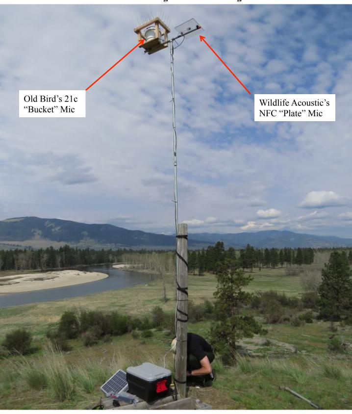
Gus designed a new mast that allows us to compare Old Bird's 21c microphone to Wildlife Acoustic's nocturnal flight call (NFC) microphone. Nature Sound Electronics modified the Old Bird mic to work with the Songmeter recorder. The 21c uses a method to amplify sounds that can result in two to five times as many recorded nocturnal flight calls.
