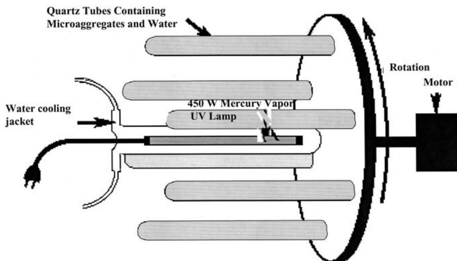
**Figure 1.** Schematic of photo-oxidation system. Microaggregates (0.2 g) are placed in horizontally oriented 50-mL DI-H<sub>2</sub>O in quartz tubes. Rotation around a 450 W mercury vapor UV lamp gently suspends microaggregate particles while tubes are irradiated from all sides.
